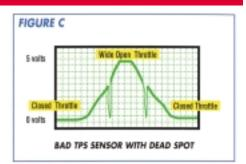
Check for the proper reference voltage between the TPS Vref wire terminal and ground with the ignition on. Less than five volts indicates a wiring or computer problem. Check for a good ground connection between the ground wire terminal and ground with the key on. The reading should be less than 0.1 volt.
