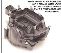
PBT, not PP. Consequently, because of differences in shrinkage rates, this cap had a slightly smaller inside diameter creating potential installation problems.
